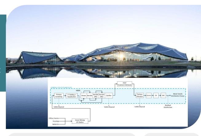
Treated roof and site stormwater is blended with onsite-treated wastewater to provided non-potable recycled water. Treatment consists of a moving bed bioreactor (MBBR) and subsurface treatment wetland. Advanced treatment includes tertiary filtration using compressible media filter, ozonation (disinfection and color removal), UV (disinfection), and organic carbon removal using GAC adsorption.
