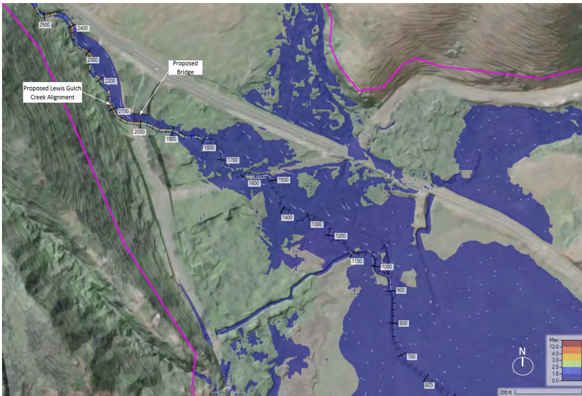
Figure 18. Proposed Conditions Plan View Q1.5 Simulation Velocity (fps) Magnitude and Distribution
